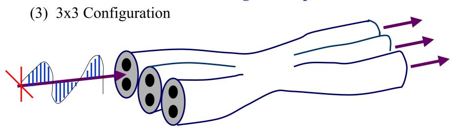
Note: It has equal splitting Ratio at any input port launched
