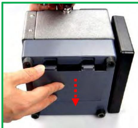
See the figure below. The lithium battery cable is connected with the power cable inside the battery case. Confirm reliable connection put the cable first into the side hole of the battery case and then install the Lithium battery. Close the battery case cover on the bottom of the fusion splicer. If replacing the lithium battery, follow the procedure above.
