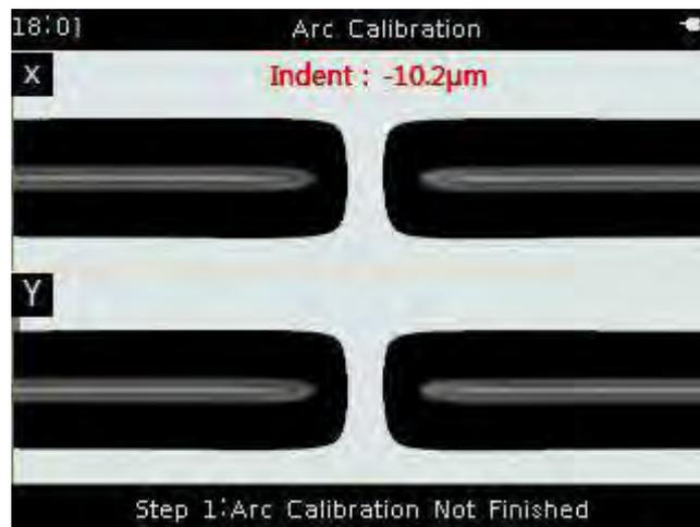
E. When "arc calibration step 1" is finished, "arc calibration step 2" is started automatically. The operator shall prepare repeatedly the fiber and let the splicer go into automatic arc calibration until the machine shows "arc calibration step 2 is finished" as shown in following figure.
